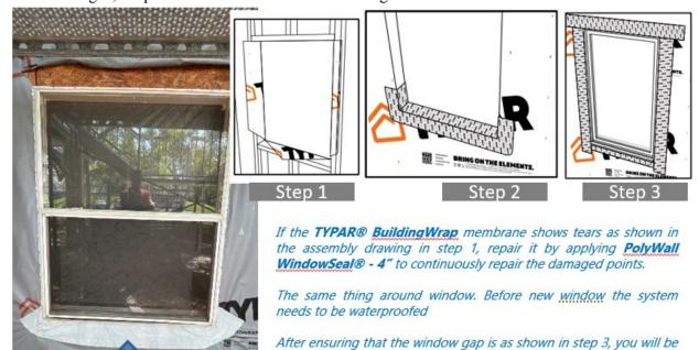
The flexible 9" flashing installed on the beam below the window must be intact, or be reinstalled (step 2)
